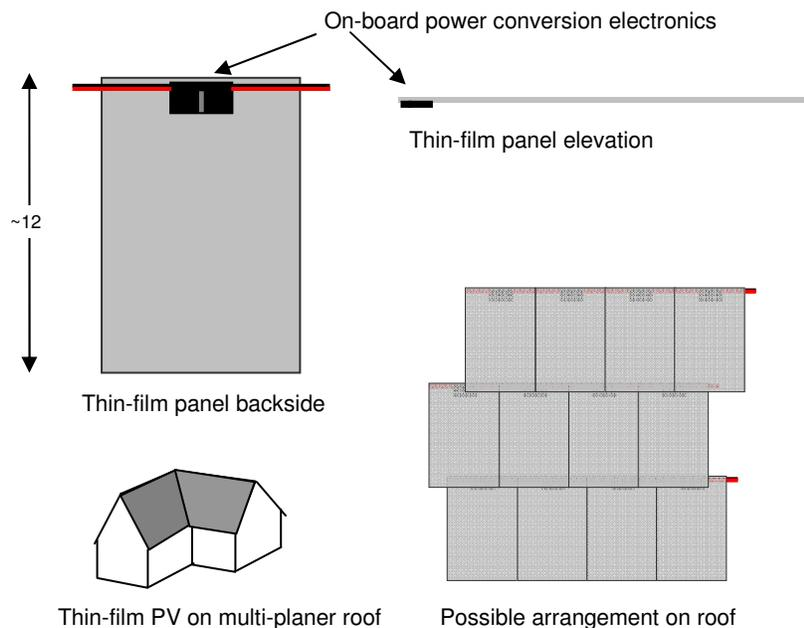
**Figure 2:** Future thin-film PV panels with on-board power conversion electronics.
